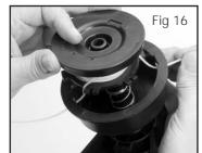
Once the spool is in place, apply pressure on the spool compressing the spring. Pull each end of the line sharply to unlock the line from the slots. Continue to apply pressure to the spool until the knob can be threaded clockwise onto
